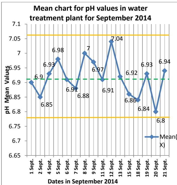
Figure 4: Mean chart for pH values in water treatment plant for September 2014.
