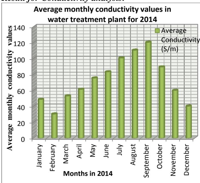
Figure 6: Average monthly conductivity values in water treatment plant for 2014.
