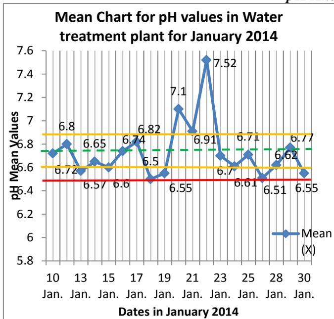
Figure 3: Mean Chart for pH values in Water treatment plant for January 2014.
