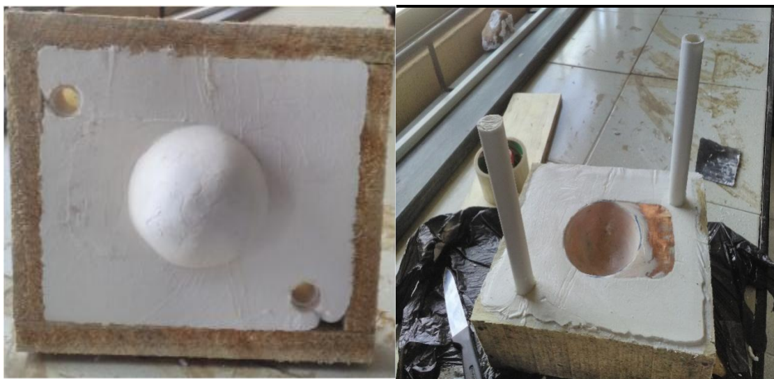
Figure 11: Mould used for the development of the helmet prototype (Cope and Drag)
