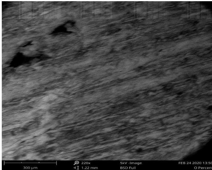
Plate 1: Microstructure of as-cast Al-3.5%Cu-0.8%Mg alloy (control sample) x300
