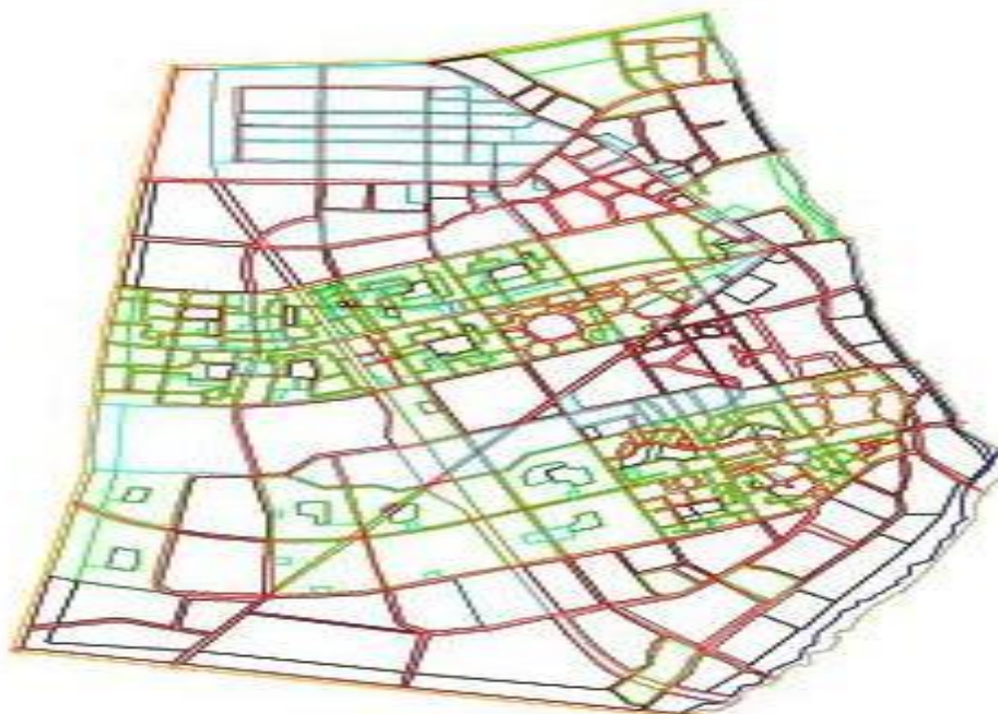
Fig. 4.3: Digitized map of new Owerri in an AutoCAD environment
