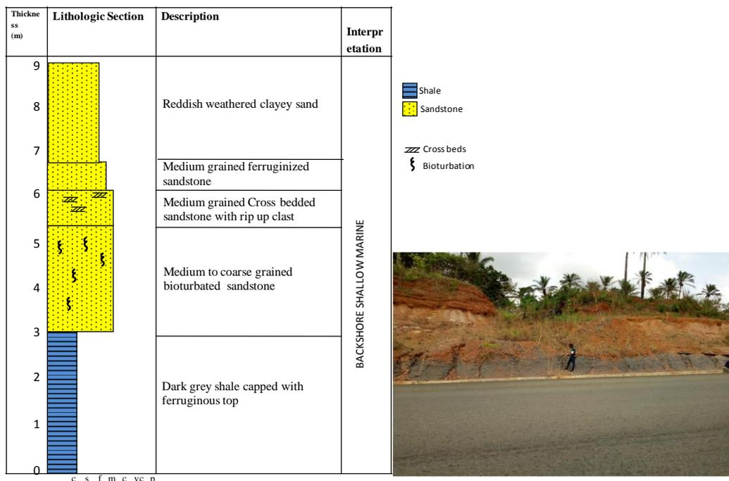
Fig 4. Litholog of section at Leru-Isuochi road
