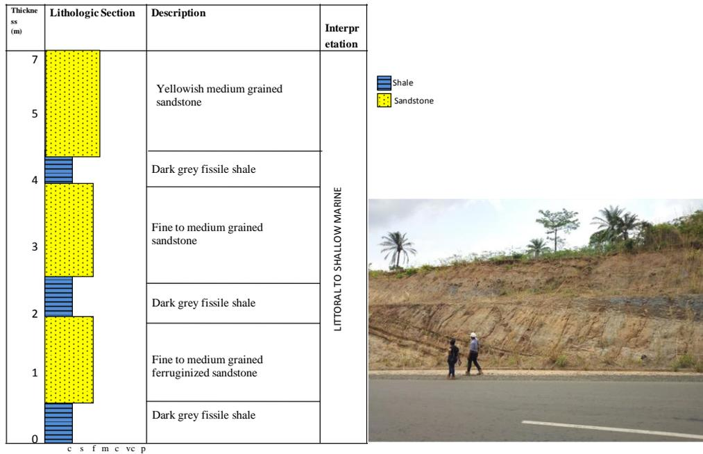
Fig 5: Litholog of section along Mmaku-Mgbidi road
