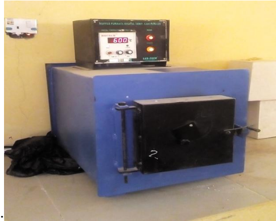
Fig. 4: The electric furnace for thermal resistance test
