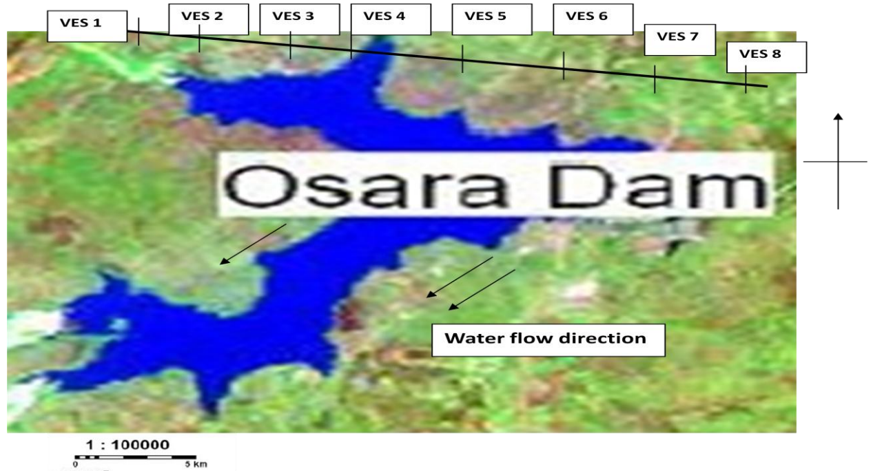
Figure 3; Data acquisition map around the dam site
