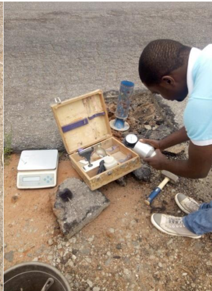
Fig 4: Performing Field Relative Density and Moisture Content Test
