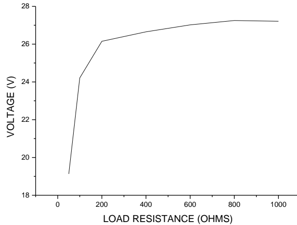
Figure 10: A curve showing the relation between the varying resistance of the applied load and the output voltage in the 30VDC range.
