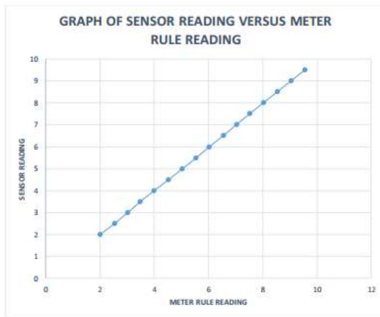
*Figure 3: Graph of Sensor's reading versus Meter rule reading using Excel*
