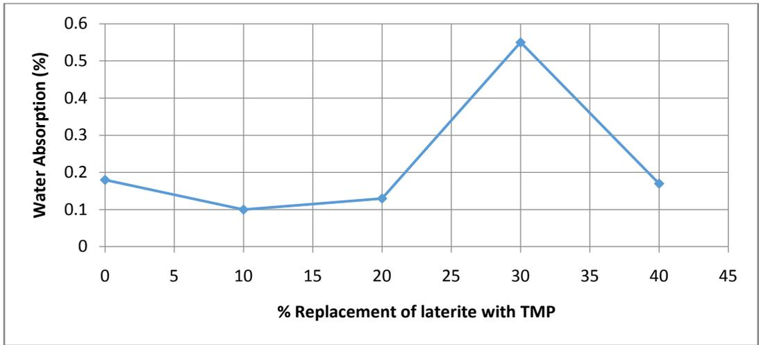
**Figure 3 Water Absorption of TMP stabilized bricks**
