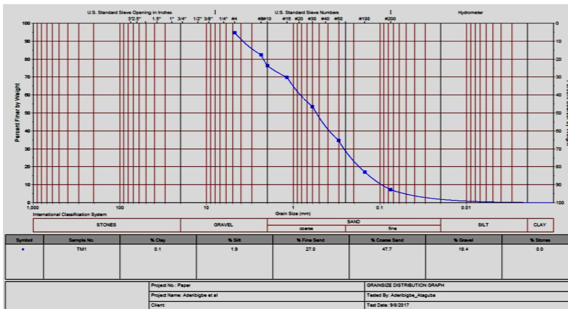
**Fig. 1: Particle Size Distribution Test Result Graph**
