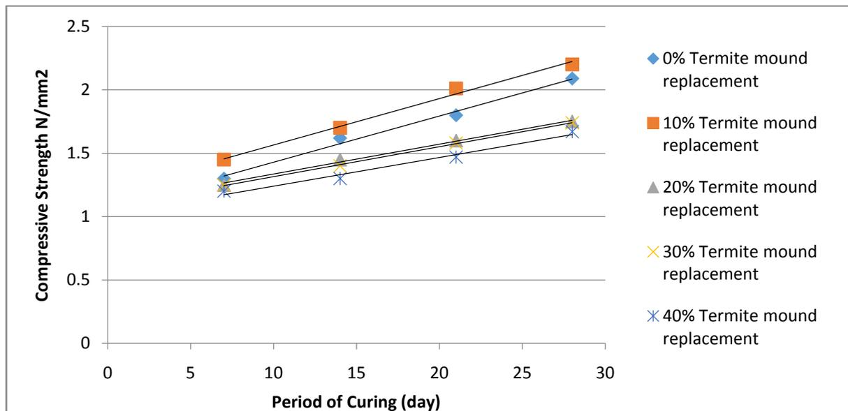
**Fig. 2 Compressive strength of TMP stabilized bricks.**
