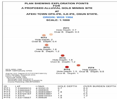
Fig. 4: Exploration plan of the sampled pits
