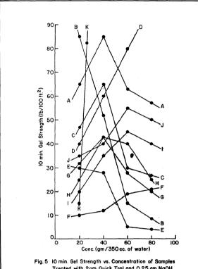
Fig. 5 10 min. Gel Strength vs. Concentration of Samples Treated with 2gm Quick Trol and 0.25 gm NaOH
